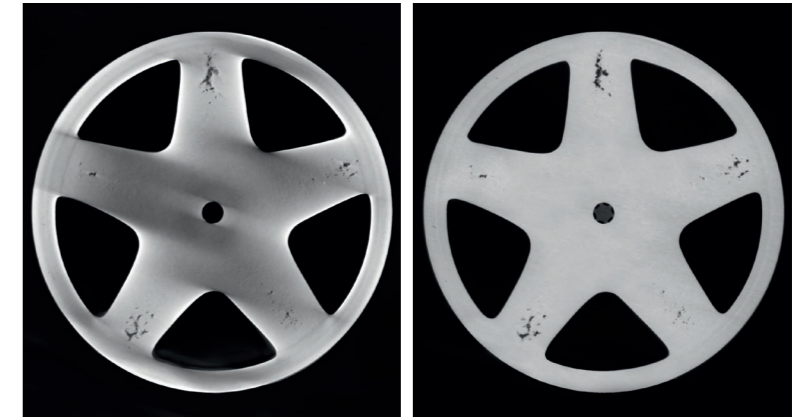
Eliminating unwanted gray-value gradients: Cone-beam CT without (left) and with Beam Hardening Correction (right).
